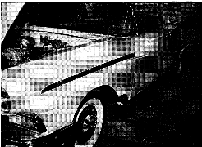
(9) Outside trim and other accessories are installed.
